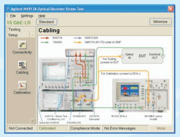
5 The setup has to be calibrated before any testing can be done. Select Calibration from the list menu given on the left side of the window. Click 'Start' to perform calibration.
